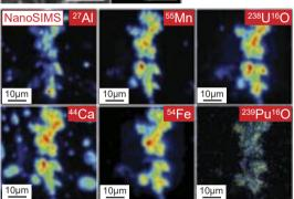
SEM-EDS is used to detect major elements. TEM permits nm-level structure analysis. Thanks to its **unique imaging sensitivity**, the NanoSIMS delivers elemental maps which reveal that amorphous iron oxide colloids adsorb Pu(IV) hydroxides or carbonates along with uranium carbonates.
