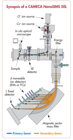
All options are field-retrofittable (charge compensation, SEM detector, multiple FCs, ...).
