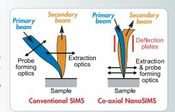
The double focusing Mattauch-Herzog-like geometry and optimized transfer optics guarantee high transmission at high mass resolution, required for analysis of small volumes of complex materials.
